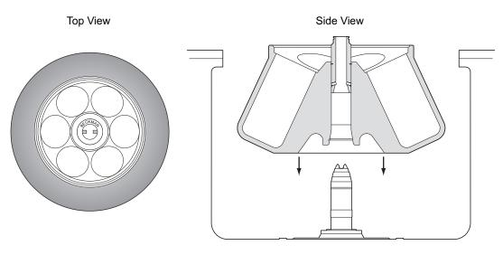
Figure 4. Installing the Rotor
