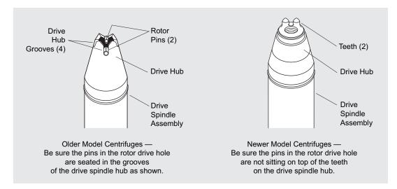
Figure 3. Centrifuge Drive Spindle Hub Configurations
