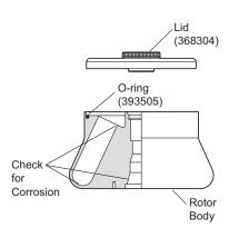
Do not use sharp tools on the rotor, as they can scratch the anodized surface. Corrosion begins in scratches and may open fissures in the rotor with continued use.
