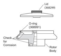
(frequently aluminum oxide), or heavy discoloration. If any of these signs are evident, do not run the rotor. Contact your Beckman Coulter representative for information about the Field Rotor Inspection Program and the rotor repair center.
