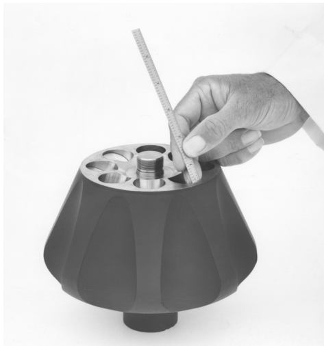
Figure 3 Measuring Distance from Cap to Rotor Tray
